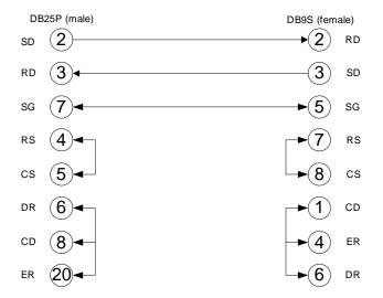
FG: Frame groundRS: Request to sendSG: Signal ground
